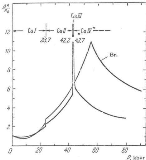
FIG. 2. Dependence of the electrical resistance of Cs on pressure.<sup>[22]</sup> The pressure scale should be corrected for Bridgman's curve (Br):<sup>[31]</sup> 100 kbar on the old scale corresponds to 80 kbar on the new scale.
